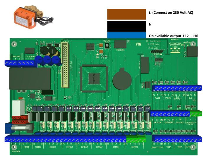
Mount the 3-way valve on the flow from the boiler.
